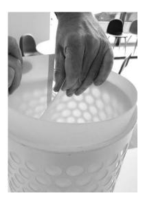
5. The new inner shade is now ready to be inserted in the lamp with the adhesive tape pointing inward
