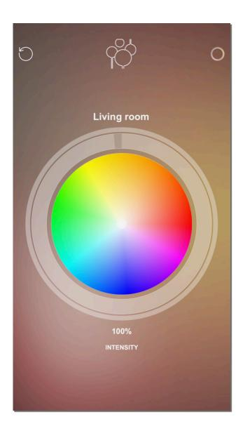
If you press on the group, you will access to the group management page. Through this page it is possible to set the intensity, the colour, or the colour temperature of the lamps that have been part of the group, by using a single control interface.
