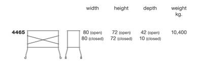
**Material** PMMA trays and chrome steel structure
