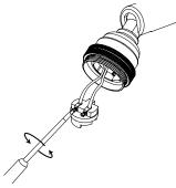
**4.** loosen screw in bottom of the holder.
