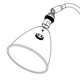
2. Press the metal flap (a) with a thin screwdriver, while screwing off the holder.
