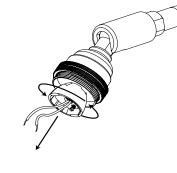
6. Insert the first part of the new lamp holder and tighten screw.
